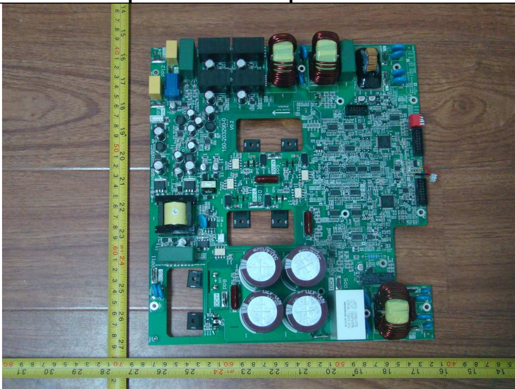
Main power board component side view
